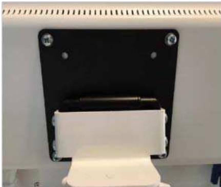
After the monitor stand is installed on the Cart, attach the LCD to the stand. A Phillips Head or (if added security is needed for the LCD) Torx Head driver is needed to attach the LCD to the VESA Stand, 4 places. Both Phillips and Torx screws are provided. It is recommended that one person hold the LCD while a 2nd person inserts the hardware. Make sure all 4 screws are installed and tightened properly.
