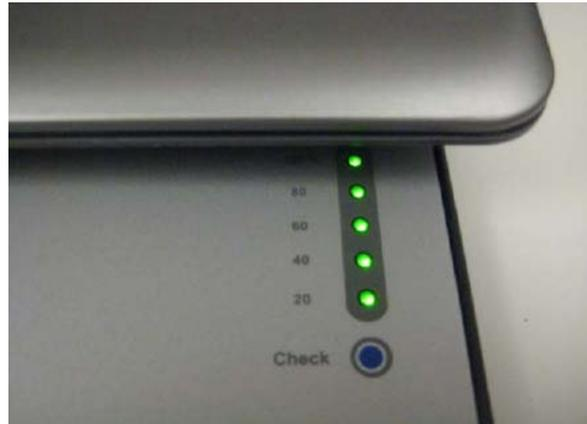
The battery is not shipped fully charged, plug in the Cart before using and allow battery to fully charge. When the battery is low, it will “beep”. Plug the Cart power cord into any 120vac wall outlet to silence the “beep” and charge the battery. During the charge, the battery status lights will blink as the charge progresses and once completely charged, all five lights will shut off.
