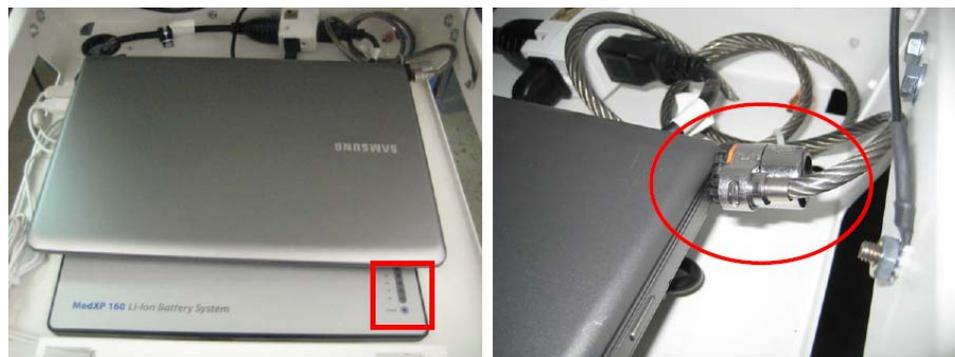
To check the battery charge status, press and hold the “Check” button on the battery.
