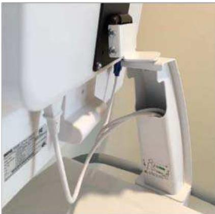
With the monitor and stand installed on the Cart, the LCD power and signal cables can be installed. Route both cables down through the cable management area of the stand as shown to the left. Pull the cables into the Top Assembly and attach to the PC or laptop computer that will be installed later.
